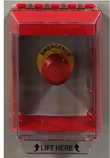
After the condition necessitating the emergency stop has been rectified, a qualified operator may reset the Emergency Stop by pulling the red button outwards and twisting the knob in a counterclockwise direction.
